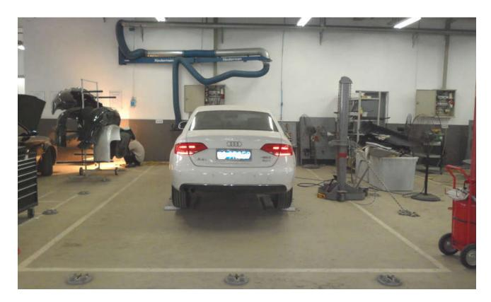
**Features:** Floor fixing system which a kind of necessary useful auto collision repair equipment.
