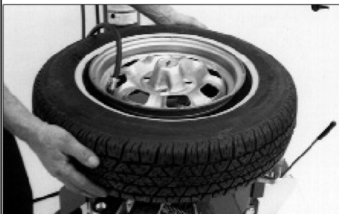
Figure 19 - Lift Tire Upwards for Bead Sealing
