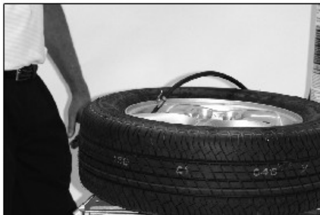
Figure 20 - Stand Back during Bead Seat
