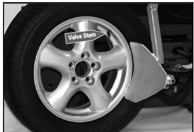
Figure 3 - Position Tire and Bead Loosener Shoe
